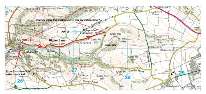
This required all residents to the east of the closure to travel up to Springhead, Water Hill then turn into Higher Lane to return down to the village centre and/or gain access to the main road network. The other option was to continue up Bushes Lane to the A3052 at Heathfield Cross.
